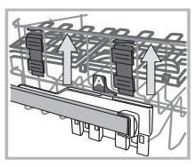
If the rack is equipped with a **Lift-Up device**\* (see figure), lift it up by holding its sides. To restore the lower position, press the levers (**A**) at the sides of the rack and follow the rack down.
